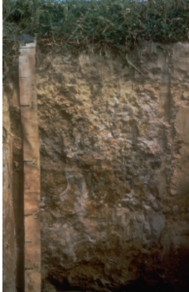
Figure 27. This is a somewhat poorly drained soil with a predominantly gray matrix starting at 0.35 m (15 in.)
