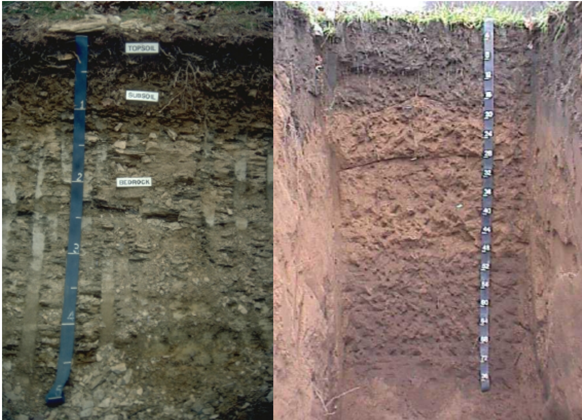
Figure 22. The soil on the left is a shallow soil with bedrock starting at 0.35 m (15 in.). The soil on the right is a very deep soil with no bedrock to a depth greater than 1.5 m (60 in.)
