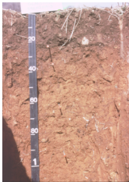
Figure 25. This soil is a well drained soil with no redoximorphic features in the upper 1 m (40 in.)
