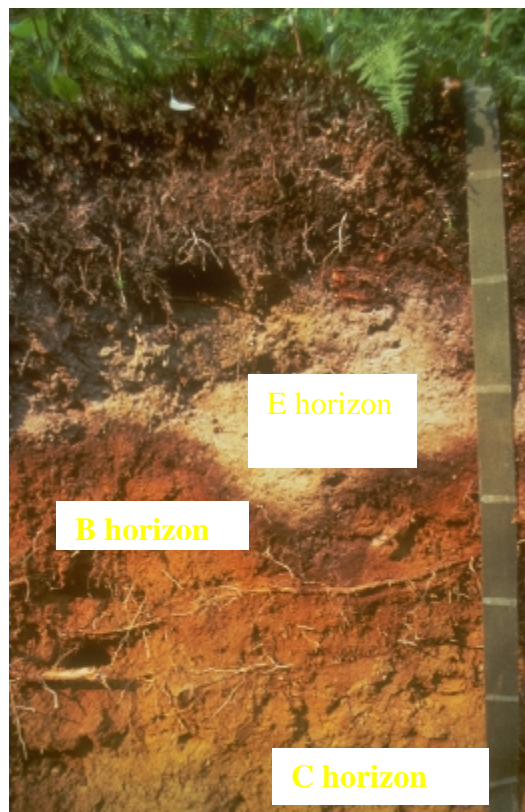
Figure 8. This profile is a soil found in the Appalachian Plateau showing an E horizon from 20 to 35 cm (8 to 14 in.) and a B horizon from 35 to 55 cm (14 to 22 in.) Measuring tape is in 10 cm increments. Below 55 cm (22 in.) is a C horizon.
