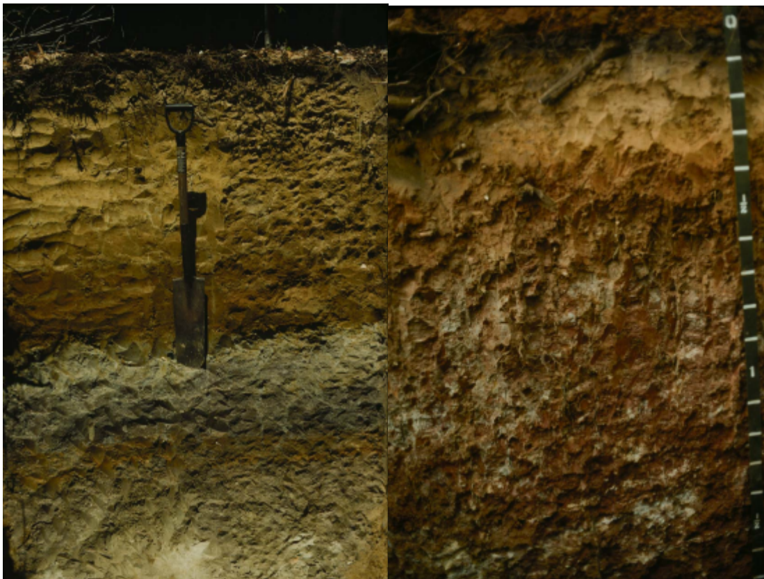
Figure 13. The red and gray colors in these soil profiles are due to wetness. These splotches of colors due to wetness are called redoximorphic features. The soil profiled and the left has a predominance of gray due to the loss of iron starting close to the bottom of the spade. The soil on the right has a predominance of red with gray splotches starting at 1 m (40 in.). The measuring tape for the profile on the right is in meters.
